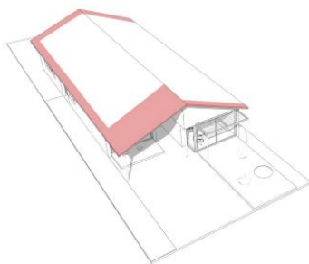
Concept sketches of key principles – design shaped to maximise northern exposure and preserve pleasant outdoor spaces, and various features used to shade windows from the summer sun.
