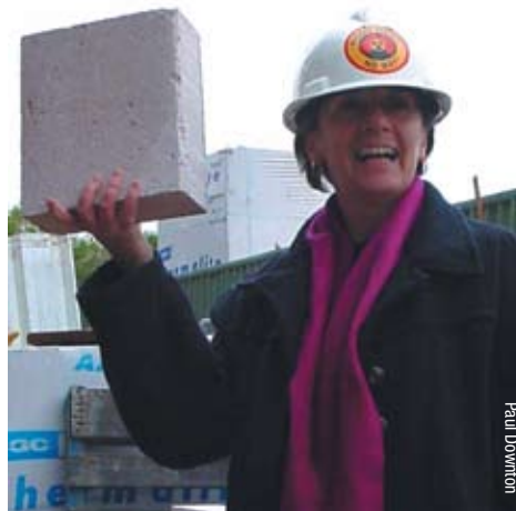
Autoclaved Aerated Concrete is about one-fifth the density of normal concrete blocks.
