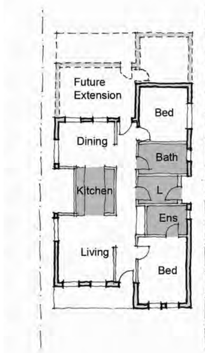
Another floor plan (above) provides larger wet areas for improved accessibility, and these wet areas are located to allow for future extensions with only minor changes to the existing dwelling.
