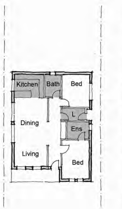
A typical house plan (above) often requires the expensive relocation of wet areas such as bathrooms and kitchen if the house is to be extended.
