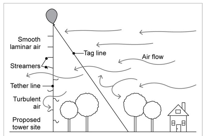
Test for smooth laminar air with a balloon, tag lines and a tether line.
